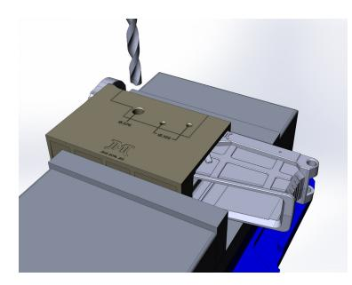
FIRMLY CLAMP THE ASSEMBLED LOWER RECEIVER AND JIG ASSEMBLY INTO YOUR VISE AS SHOWN AND SECURE TO THE TABLE OF YOUR MILL OR DRILL PRESS. VERIFY THAT THE SURFACE OF THE JIG IS LEVEL IN THE X AND Y AXIS.
