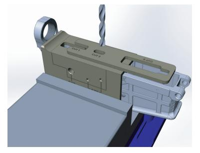
USING THE 5/16" dia. (.313) drill bit or end mill make the cut indicated in the reference drawing using the slot labeled cut 3 in the Jig top plate as a guide.
