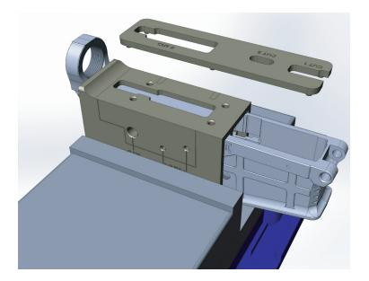
REMOVE THE JIG TOP PLATE FROM THE ASSEMBLY, ROTATE THE TOP PLATE 180 DEGREES AND REINSTALL. TAP THE JIG TOP PLATE INTO PLACE UNTIL FULLY SEATED.
