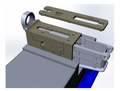
FIRMLY CLAMP THE ASSEMBLED LOWER RECEIVER AND JIG ASSEMBLY INTO YOUR VISE AS SHOWN.
