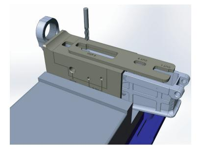
MACHINE THE POCKET SHOWN IN THE REFERENCE DRAWING USING THE 5/16" dia. END mill in the same manor as before, stepping as you go.
