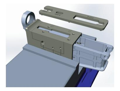
REMOVE THE TOP JIG PLATE FROM THE ASSEMBLY, ROTATE THE TOP PLATE 180 DEGREES AND REINSTALL. TAP THE JIG TOP PLATE INTO PLACE UNTILL FULLY SEATED.
