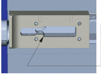
USE CARE WHEN REMOVING MATERIAL FROM THIS AREA, THIS SURFACE IS REQUIRED FOR PROPER FUNCTION WHEN ASSEMBLED
